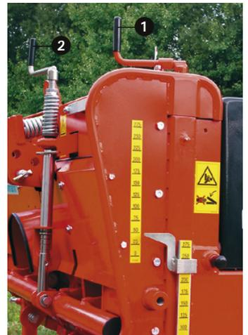
Achieve different spiking intensities by adjusting the entry angle of the tines.
