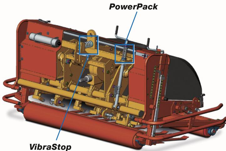
To eliminate this fundamental drawback, Wiedenmann has developed two independently operating, exclusive damping systems - **VibraStop** and **PowerPack**. Together, they absorb perfectly all jolts and vibrations caused by extreme compaction or stones. The result is unrivalled smoothness of running with a minimum of strain on the driver, tractor, deep aerifier and tools.
